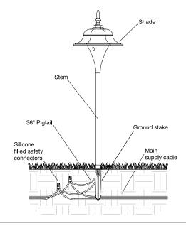
The operating voltage range for this LED luminaire is 6 - 15 volt AC. The Vista electronic driver ensures the LED operates at the intended lumen output while receiving voltage as low as 6 volts, and as high as 15 VAC, resulting in a balanced lumen output from the first fixture to the last. Eliminating the dimness issues often attributed to voltage drop.
