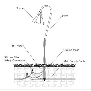
The operating voltage range for this LED luminaire is 6 - 15 volt AC. The Vista electronic driver ensures the LED operates at the intended lumen output while receiving voltage as low as 6 volts, and as high as 15 VAC, resulting in a balanced lumen output from the first fixture to the last. Eliminating the dimness issues often attributed to voltage drop.
