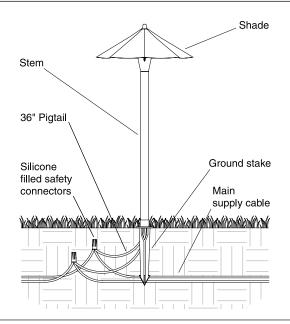
The operating voltage range for this LED luminaire is 6 - 15 volt AC. The Vista electronic driver ensures the LED operates at the intended lumen output while receiving voltage as low as 6 volts, and as high as 15 VAC, resulting in a balanced lumen output from the first fixture to the last. Eliminating the dimness issues often attributed to voltage drop.
